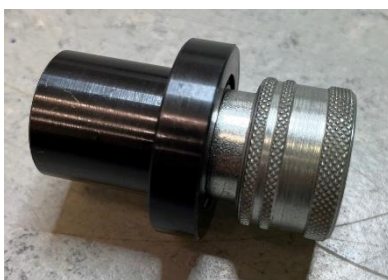
Foto 02: Module unit with sliding sleeve
